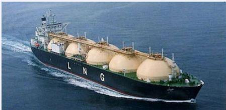
**Shipping:** The typical LNG carrier can transport 125,000 to 138,000 cubic meters of LNG, which will provide about 2.6 to 2.8 bcf of natural gas. The typical carrier measures 900 feet in length, 140 feet in width and 36 feet in water draft, and costs about \$160 million.
